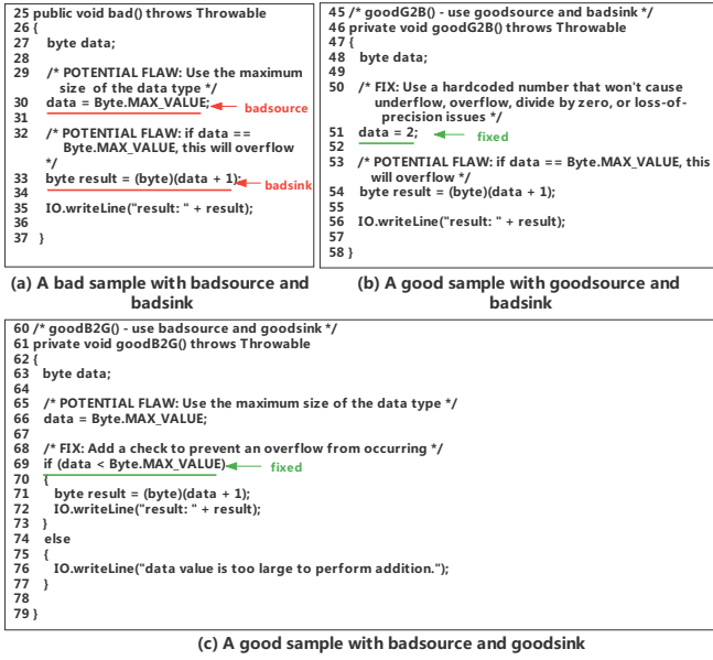
Fig. 2: The source code of samples extracted from the test case 128562 in Juliet.
